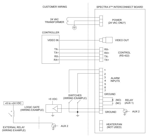
Figure 8. Wiring Diagram for Spectra II™
